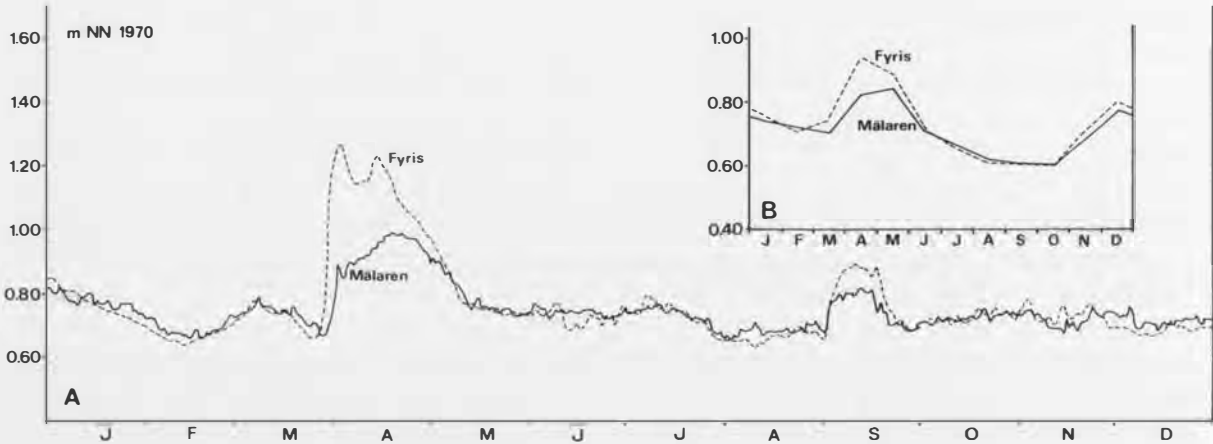
Fig. 15. The daily water levels (A) for 1978 and the monthly mean water levels (B) for the period of 1968–1980 in the River Fyris at Ultuna and in Lake Mälaren (mean value recorded at KJ. Slussen, Södert. Slussen and Västerås Hamn). The water level is expressed in m above sea level in system 1970. The data for the River Fyris obtained from Anders Bjerketorp (unpublished) and for Lake Mälaren from SMHI. Redrawn by the author.
